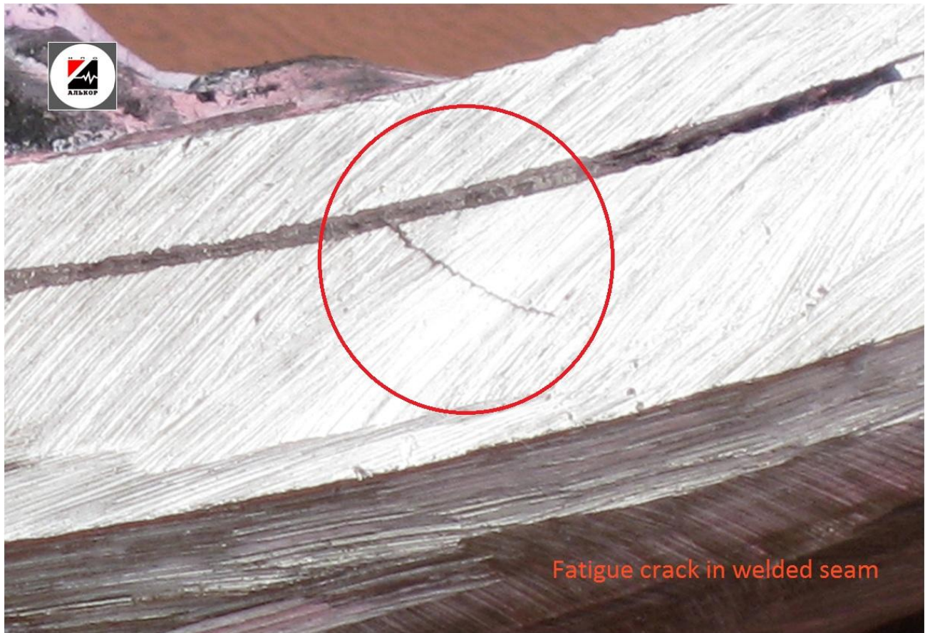
Fig. 5. The fatigue crack which has been found out ISHM «Pecypc-2000» in a welded seam of the refinery pipeline.
